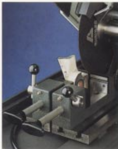
T-slot work table with dual cam-activated vises secure samples during sectioning. Optional T-slot Clamping Kit accommodates irregularly shaped samples.
