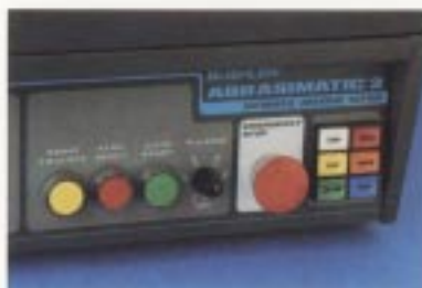
Front panel mounted controls allow operator to choose between continuous or pulse feed cutting modes.
