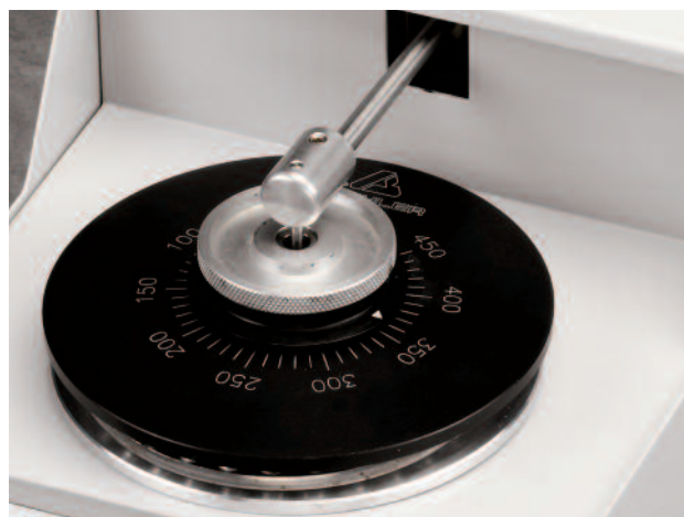
Precision Thinning Attachment enables SEM and TEM samples to be prepared.
