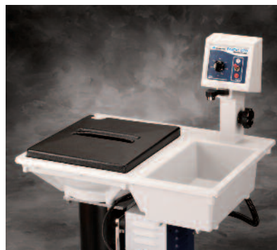
The cover keeps debris away from the platen when not in use.
