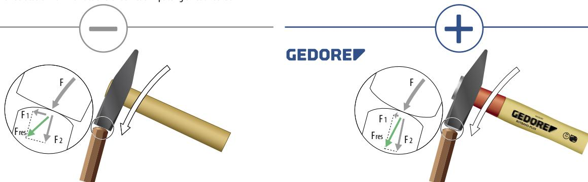
GEDORE hammers and chisels are optimally adapted to each other. Their regulation-compliant geometrical shape diverts the bulk of the forces raised towards the chisel tip.
