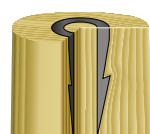
several hundred strikes. The barbed hook ensures a positive fit and stops the tapered collar from loosening. A safety "extra".
