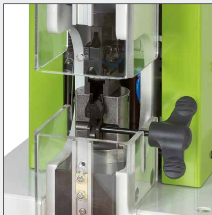
CM 25-2 crimping machine for processing shielded modular connectors
