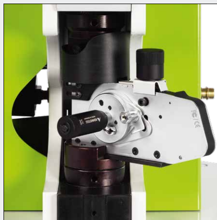
Crimping unit with universal locator for industrial contacts
