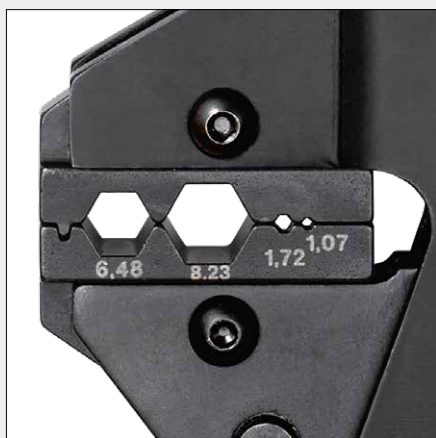
Replaceable crimp insert
