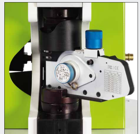
Crimping unit with single locator for aviation contacts
