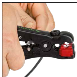
Trimming coax cables
