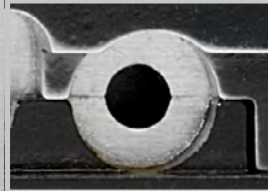
Stripping Area (Round Blades, no wire damage)
