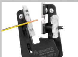
Automatic stripping of the insulation.
