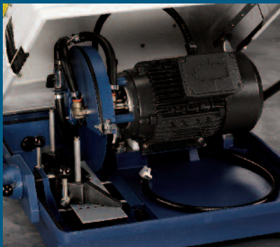
Delta® PetroCut™ Cutter showing Rock Clamp Assembly and Clean-out Hose.
