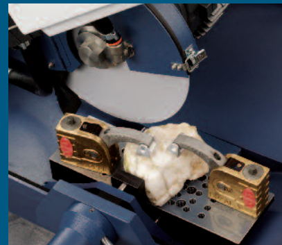
Optional Speed Vise Accessory Kit allows increased flexibility when clamping irregular shapes.
