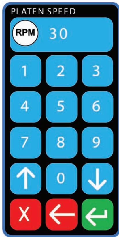
Numerical pop-up key pads allow input of parameters such as platen speed, time and force.
