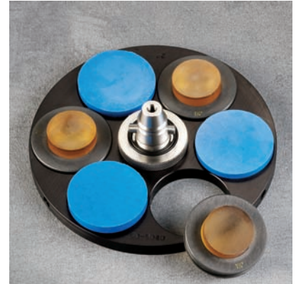
Distance ring specimen holders accommodate a variety of different sample sizes (single force only).
