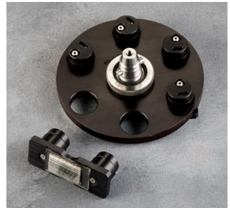
Glass slide holders connect to specimen holder with unique clamping design.
