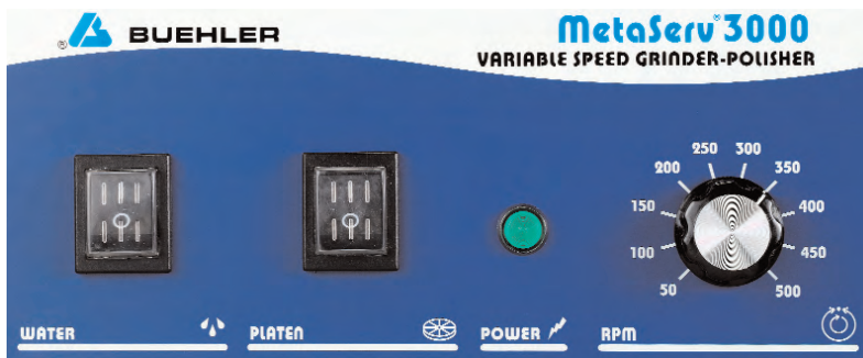
The MetaServ® 3000 front panel feature Water On/Off Control, Platen On/Off Control, Variable Platen Speed RPM Control and a green LED Power On Indicator.
