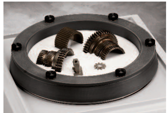
Large mounted specimens may be polished with ease. Once loaded, specimens require little operator attention.
