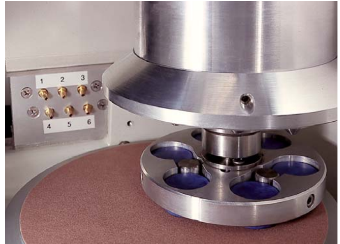
Buehler Vanguard 2000 system gives the operator the choice of preparing samples using single or central force application. Single force application means as few as one or as many as six samples can be prepared at a time. With single force application, individual samples can be removed, examined, then returned to the holder to continue preparation.
