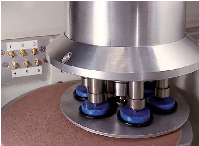
Buehler Vanguard 2000 system gives the operator the choice of preparing samples using single or central force application. Single force application means as few as one or as many as six samples can be prepared at a time. With single force application, individual samples can be removed, examined, then returned to the holder to continue preparation.
