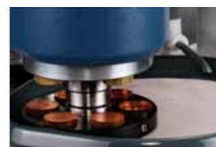
The Vector Power Head gives the operator the choice of preparing samples using single or central force application.
