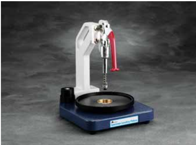
The 60-2410 Specimen Loading Fixture and 60-2413 Specimen Loading Plate level the specimens within the holder.
