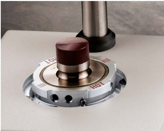
Hot compression mounting produces a reliable and consistent specimen mount.
