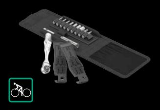
14-piece set, in a pouch; 1 Wera Bit Ratchet Zyklop Mini 1, drop-forged full steel design, suitable for ¹/₄" hex bits as per DIN ISO 1173-C 6.3 and E 6.3 and Wera series 1 and 4; can also be used with ¹/₄" sockets by using the Wera socket adaptor 870/1; 1 universal bit holder (100 mm), stainless steel, retaining ring, and strong permanent magnet; 10 bits, tough, for universal use; 1x 9502 tyre jack with bit mounting, 1x tyre jack with valve ejector.
