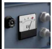
Our screwdrivers are tested for dielectric strength under a 10,000 volt load to make sure that their most important property, their insulation, has been exhaustively tested. Each individual Wera VDE screwdriver is subjected to this test to guarantee safe working up to 1,000 volts.
